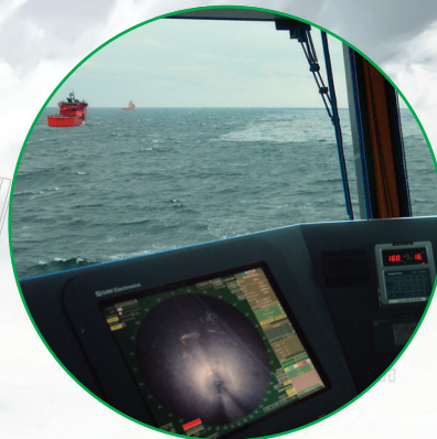
FIG:3 – OSD Monitor in the foreground displaying oil spill that can be clearly seen outside from the ship's bridge.
